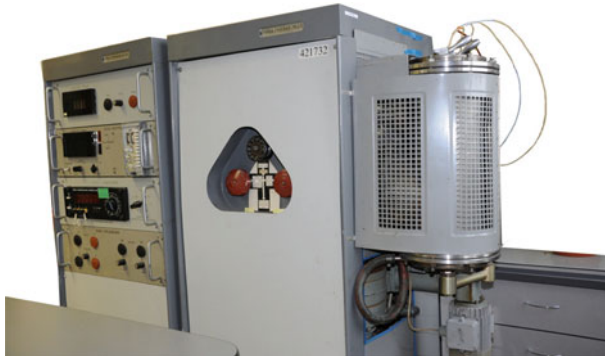
Fig. 3 Exterior view of the measuring system used for the “wire-by wire” calibration (components of the measuring system are the vertical vacuum furnace, power supply, and control unit)
